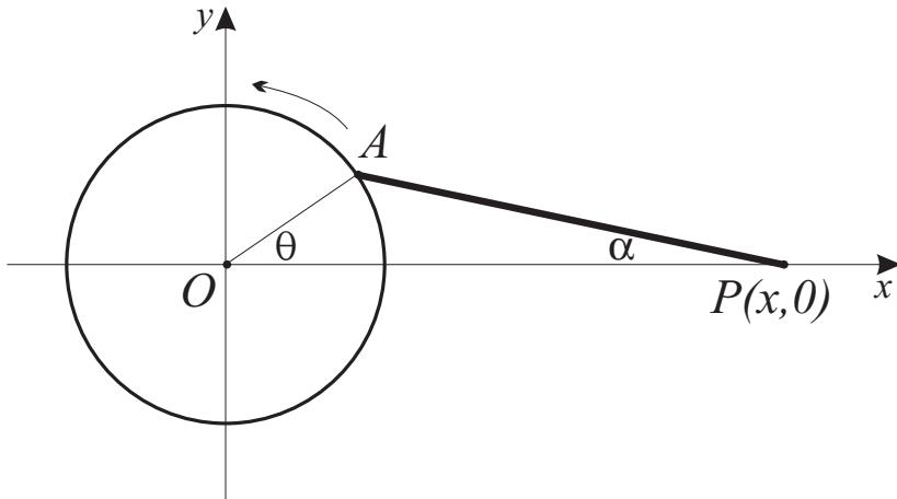
The diagram above shows a rotating wheel with radius 40 cm and a connecting rod  $AP$  with length 120 cm. The pin  $P$  slides back and forth along the  $x$ -axis as the wheel rotates anticlockwise at a rate of 6 revolutions per second. In each part below you need only address the case where  $A$  is in the first quadrant.
